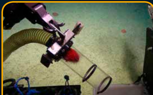
Life at these depths can be fragile and samples must be collected with great care. We had a great piece of kit for that kind of work: the slurp gun!
